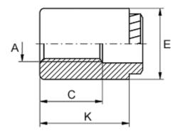
Female thread A = M3 Height K = 12 Hole diameter +0.1 = 4.2 Min distance to edge = 2.4 Min material thickness = 1.5 Outer diameter E = 7 Thread length = 9
